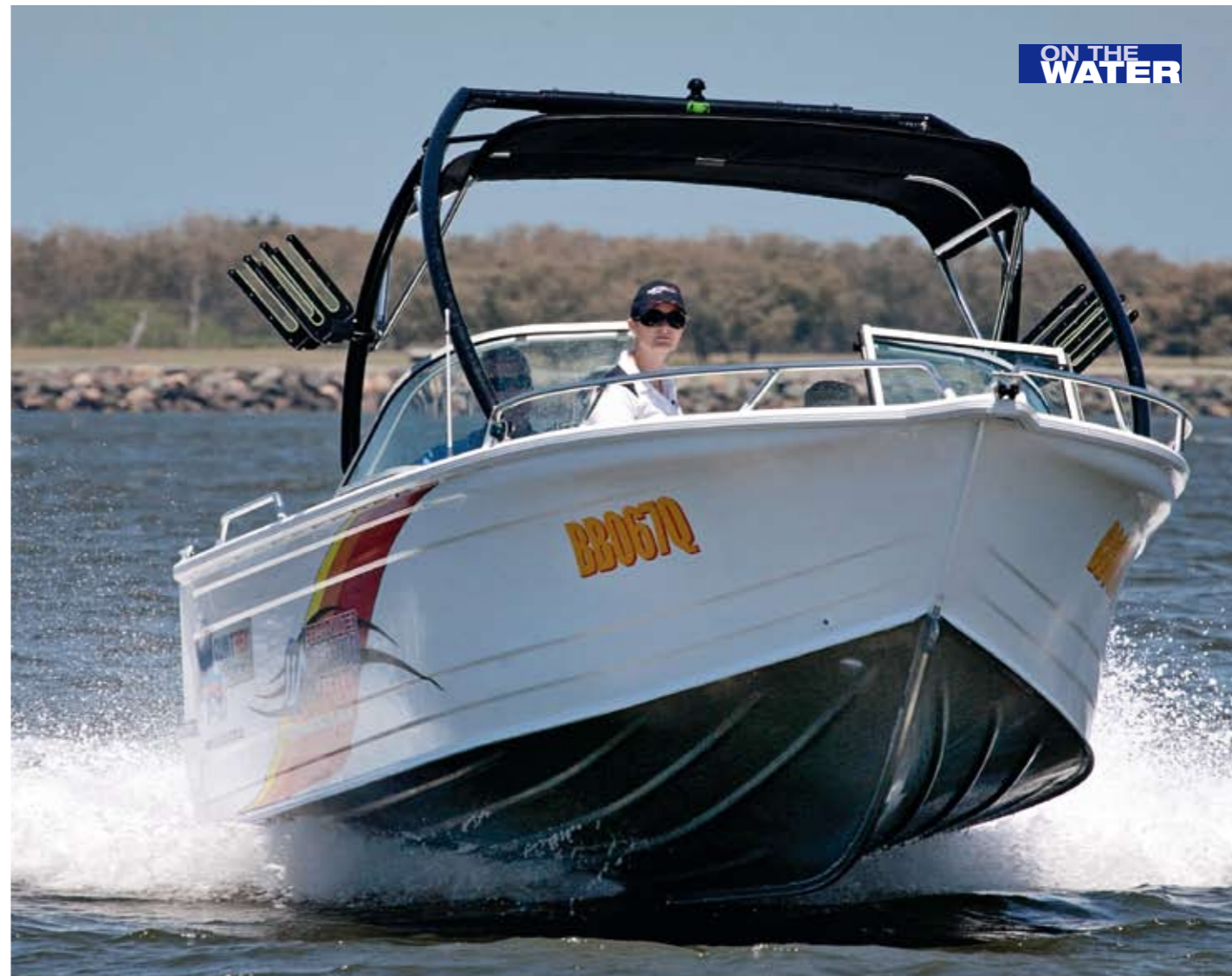
Above: With a stretch-formed, variable deadrise hull, the ride is as soft as many 'glass bowriders — yet this boat still as tough as any tinnie.
